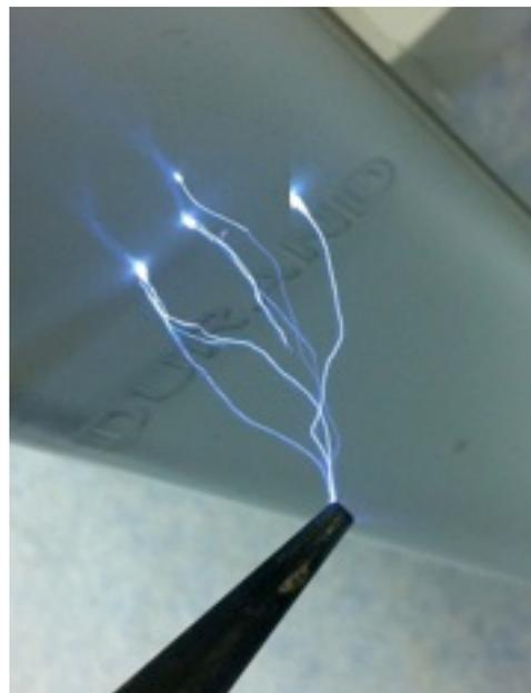
The high frequency generator is a variation of a tesla coil. It has a primary coil which produces an output voltage of about 1200 V at the input line frequency, 50 or 60 Hz. This output voltage is interrupted by a vibrating contact, energized by this coil at twice the line frequency. The output voltage of this primary coil is connected to capacitors, which are then discharged into a high voltage coil.
